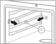
■ When replacing the runners, make sure that they are inserted correctly (see illustration). Press them in firmly.
